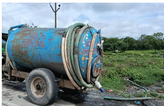
Image 6-12: Desludging vehicles queued up for discharging faecal sludge in sewer manhole
