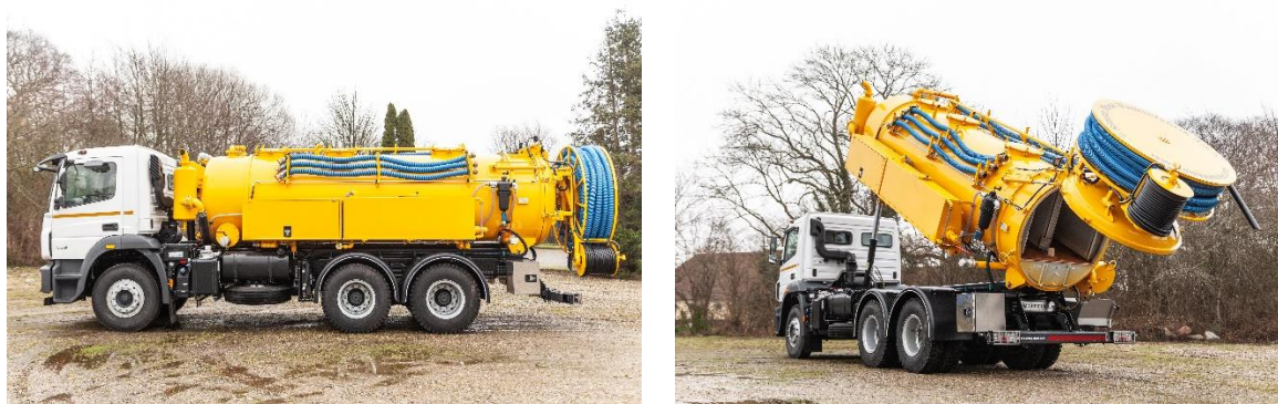
Image 6-13: Mobile Septage Treatment Unit
