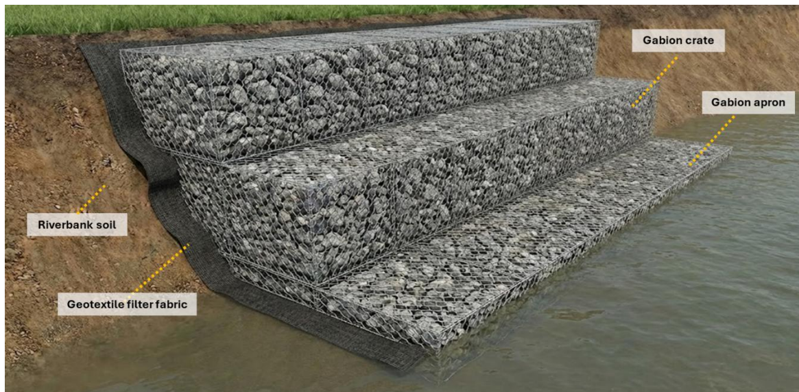
Image 6-3: Gabion bank protection measures proposed for the riparian stretch along western bank
