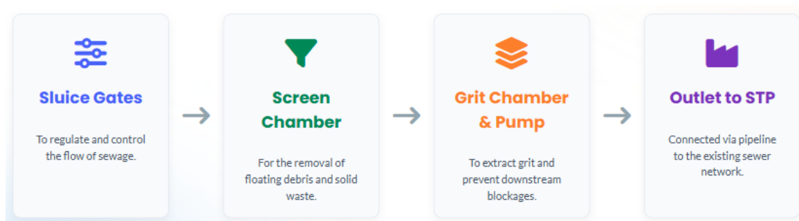
Figure 6-2: Flow arrangement of proposed I & D Structure
